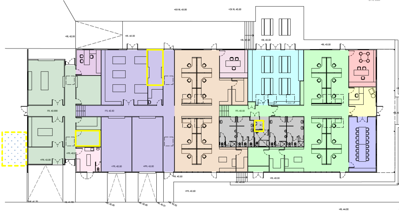
Figure 8 Waste Storage Areas at the Administration / Services Building
